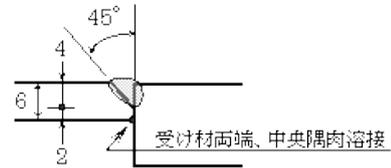
溶接部断面係数  $Z = \frac{1000 \times 6^2}{6} = 6000 \text{ mm}^3/m$
